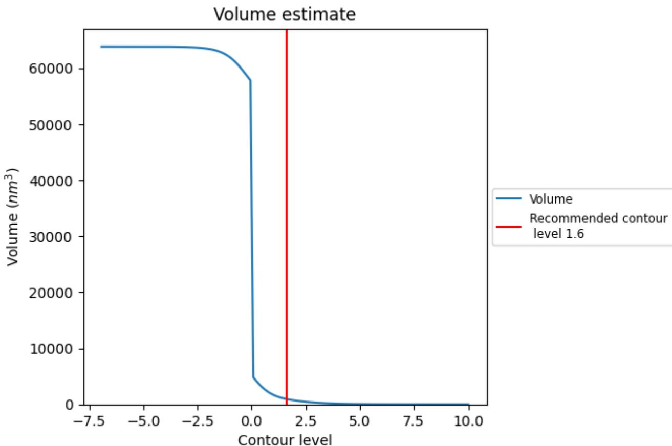
The volume at the recommended contour level is 969 nm<sup>3</sup>; this corresponds to an approximate mass of 876 kDa.
