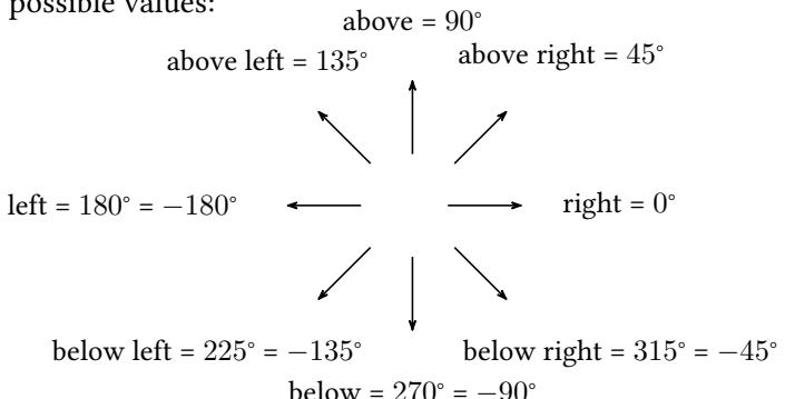
Additionally you can use every angle from the interval  $[-360^\circ; 360^\circ]$ .
