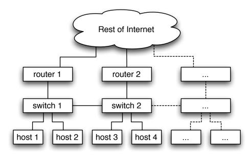
Routers and hosts communicate within a common subnet (e.g. a VLAN plumbed through some switches)
